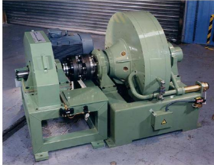
Figure No 1 Experimental set up of eddy current dynamometer
